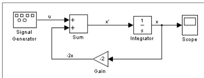
An important concept in this model is the loop that includes the Sum block, the Integrator block, and the Gain block. In this equation,  $x$  is the output of the Integrator block. It is also the input to the blocks that compute  $x'$ , on which it is based. This relationship is implemented using a loop.
