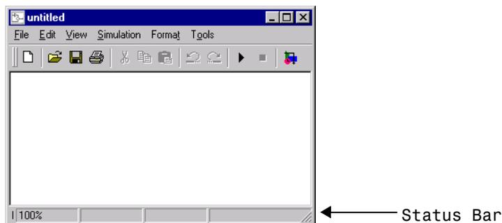
When a simulation is running, the status bar displays the status of the simulation, including the current simulation time and the name of the current solver. You can display or hide the status bar by checking or unchecking the **Status Bar** item on the Simulink **View** menu.
