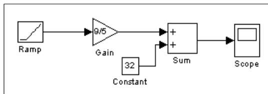
The Ramp block inputs Celsius temperature. Open that block and change the **Initial output** parameter to 0. The Gain block multiplies that temperature by the constant 9/5. The Sum block adds the value 32 to the result and outputs the Fahrenheit temperature.
