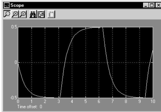
The equation you modeled in this example can also be expressed as a transfer function. The model uses the Transfer Fcn block, which accepts  $u$  as input and outputs  $x$ . So, the block implements  $x/u$ . If you substitute  $sx$  for  $x'$  in the equation above.
