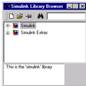
The Library Browser displays a tree-structured view of the Simulink block libraries installed on your system. You can build models by copying blocks from the Library Browser into a model window (this procedure is described later in this chapter).
