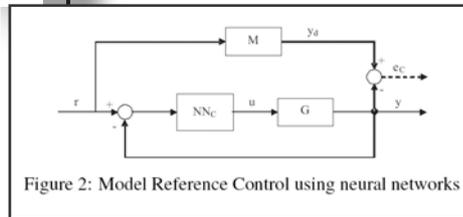
Figure 2: Model Reference Control using neural networks
