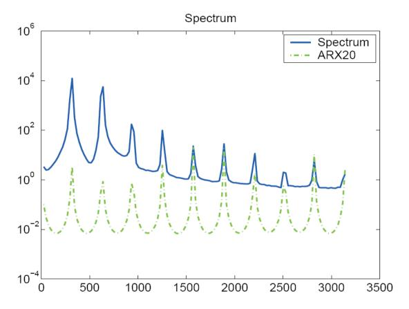
All the harmonics are now picked up, but why has the level dropped? The reason is that ARX20 contains very thin but high peaks. With the crude gitter of frequency points in the plot we simply don't see the true levels of the peaks. We can illustrate this as follows:
