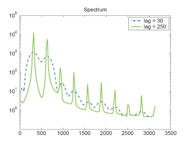
We see that a very large lag window will be required to see all the fine resonances of the signal. Standard spectral analysis does not work well.
