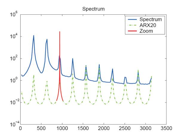
If we are primarily interested in the lower harmonics, and want to use lower order models we will have to apply prefiltering of the data. We select a fifth order Butterworth filter with cut-off frequency at 200 Hz. (This should cover the 50, 100 and 150 Hz modes).
