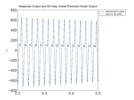
For a complete model of the signal, ARX20 thus is the natural choice, both in terms of finding the harmonics and in prediction capabilities. For models in certain frequency ranges we can however do very well with lower order models, but we then have to prefilter the data accordingly.
