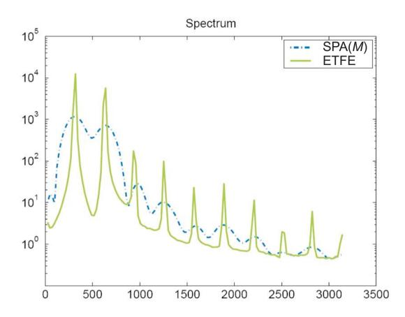
We see that a very large lag window will be required to see all the fine resonances of the signal. Standard spectral analysis does not work well. Let us instead compute spectra by parametric AR-methods. Models of 2nd 4th and 8th order are considered:
