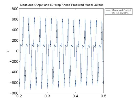
For a complete model of the signal, ARX20 thus is the natural choice, both in terms of finding the harmonics and in prediction capabilities. For models in certain frequency ranges we can however do very well with lower order models, but we then have to prefilter the data accordingly.
