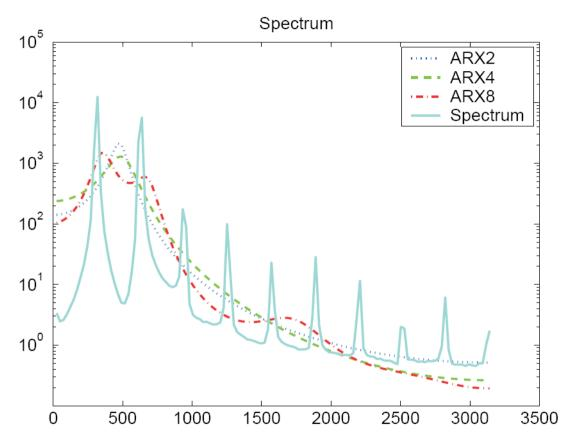
We see that the parametric spectra are not capable of picking up the harmonics. The reason is that the AR-models attach too much attention to the higher frequencies, which are difficult to model.
