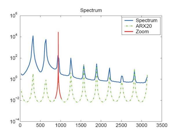
If we are primarily interested in the lower harmonics, and want to use lower order models we will have to apply prefiltering of the data. We select a fifth order Butterworth filter with cut-off frequency at 200 Hz. (This should cover the 50, 100 and 150 Hz modes). Model the lower harmonics:
