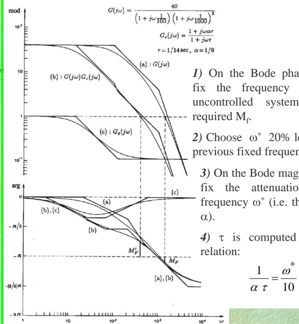
1) On the Bode phase diagram fix the frequency where the uncontrolled system has the
